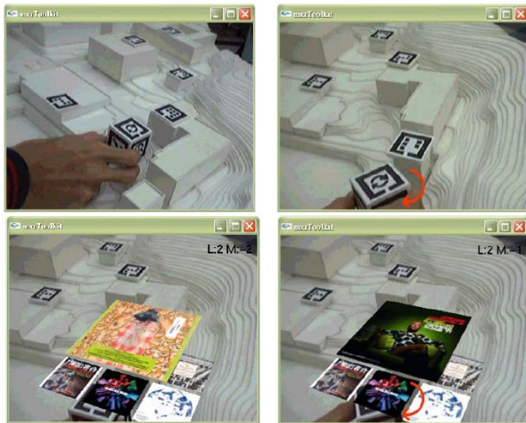
Figure 5. Media planning with tangible blocks Planners can rotate the control block to trigger and select different media
